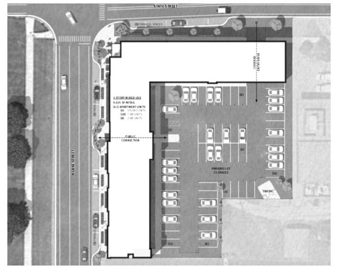
The new proposal is for a three story, 40 foot, building that includes 42 apartments, 9,025 square feet of retail space and 72 dedicated parking spaces. Courtesy image
